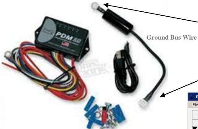
Connect your accessory ground wires (grips, GPS, 12V socket, etc.) to this end. Use the supplied bolt/nut/ring terminals to secure. If you desire, you can also use a suitable chassis ground point. (not recommended for audio/intercom)
